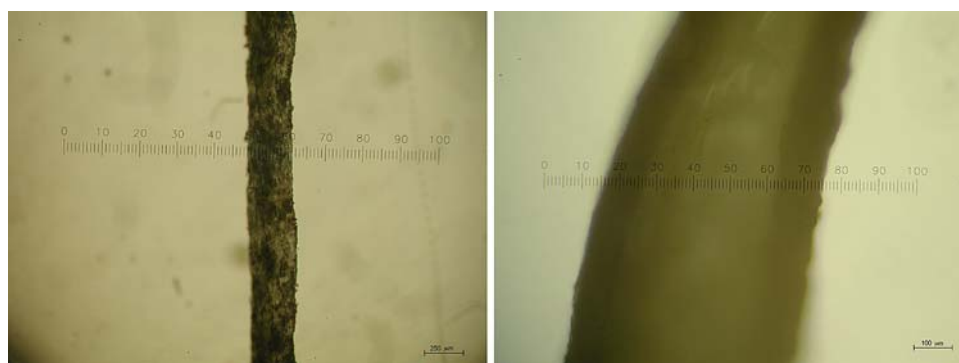
Fig. 3 Micrographs of an IPN fiber in dry (left) and hydrated states (right). The fiber was prepared from experimental condition #1 in Table 1. The scale bars represent 250 \mu\text{m} (left) and 100 \mu\text{m} (right), respectively
